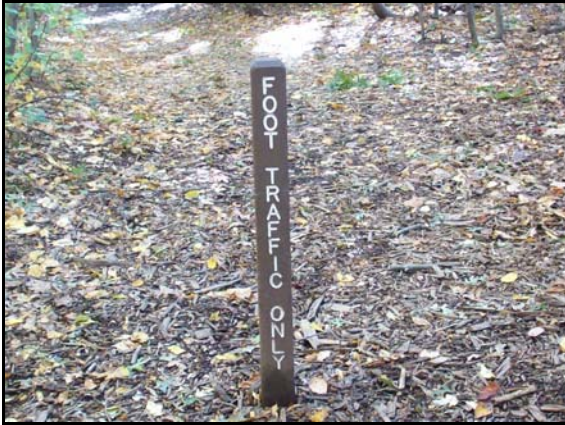
Photo 4: When tread width is less than six feet, it is appropriate to restrict the trail's use to pedestrians only.
